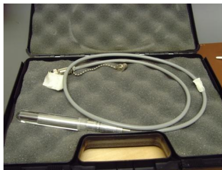
Figure 2: Farmer-type Ionization Chamber
