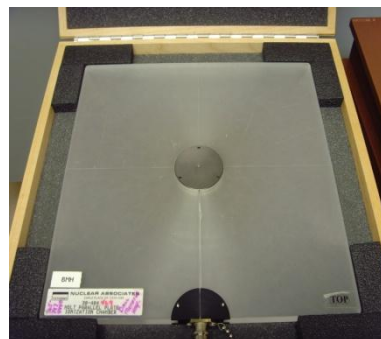
Figure 3: Parallel-Plate Ionization Chamber
