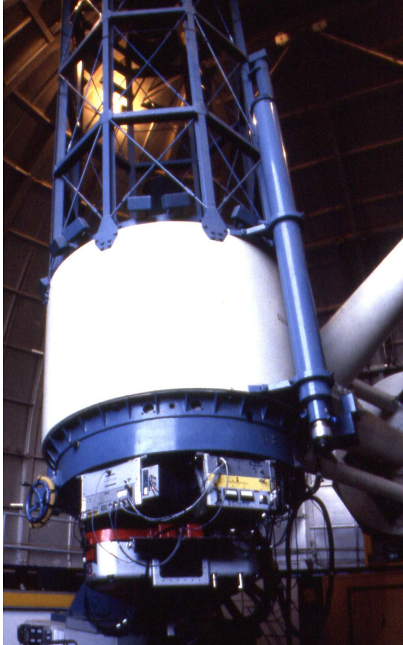
Figure 5: IDS spectrographs attached to the Perkins 1.8m (72") telescope.
